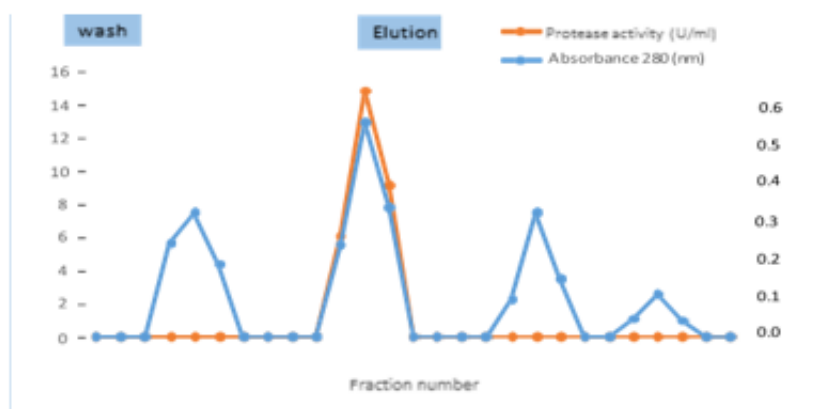
Figure 7. A DEAE-Cellulose column (45 x 2 cm) is used in ion exchange chromatography to purify the protease produced by Escherichia coli .
