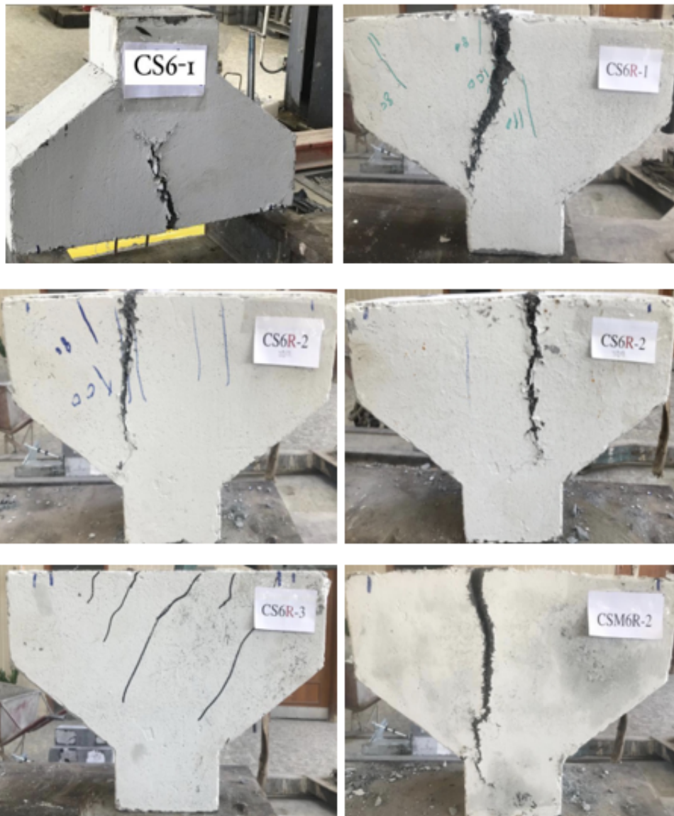
Figure 8. Failure of SIFCON corbels
