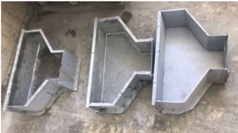
(a) Iron corbels molds
