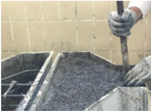
(b) Compacting with steel rod
