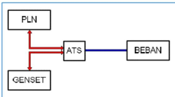
Figure 2. Blok Diagram Sistem Genset
