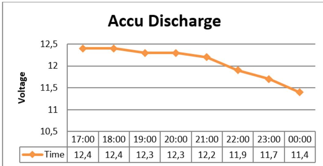
Gambar 8. Discharge Output accu
