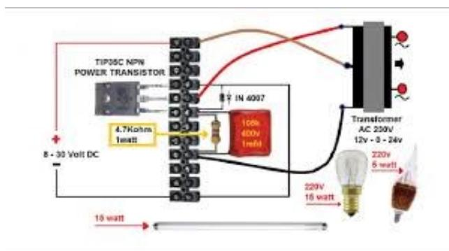
Figure 5. Rangkaian Inverter
