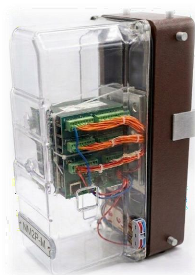
Figure 3. Installation of the developed microprocessor modules inside the existing relay block housing for experimental integration into the BRRI system.
