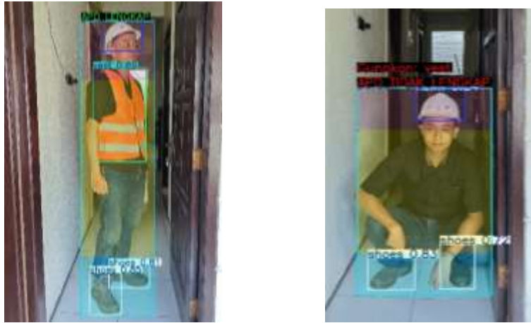
Figure 10 . Verification result: (a) Compliant worker detected with full PPE; (b) Non compliant worker detected with missing vest alert.
