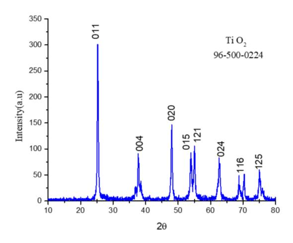
Figure 1. XRD pattern of TiO2 NPs
