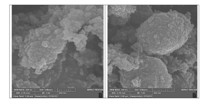
Figure 2. FE-SEM Image of TiO2 NPs
