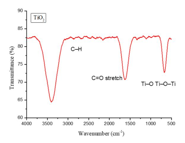
Figure 3. FTIR Spectrum
