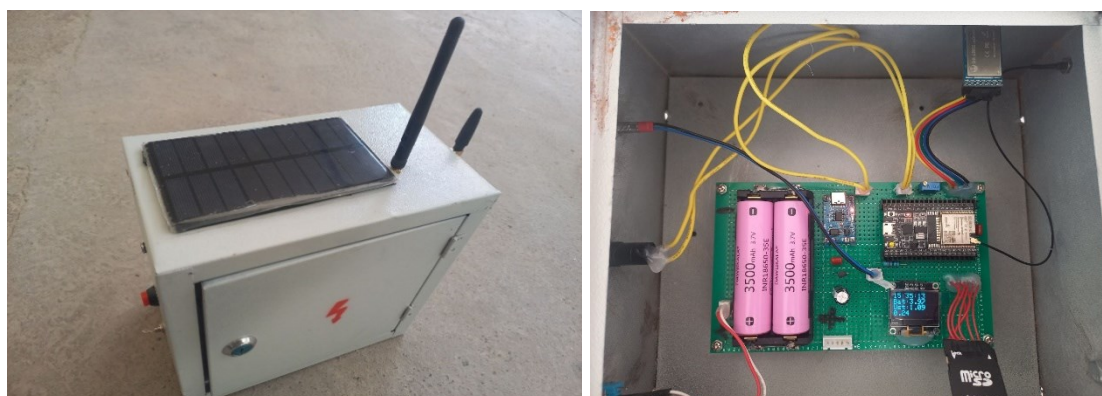
Figure 6. External view of the repeater module and the device inside the enclosure.
